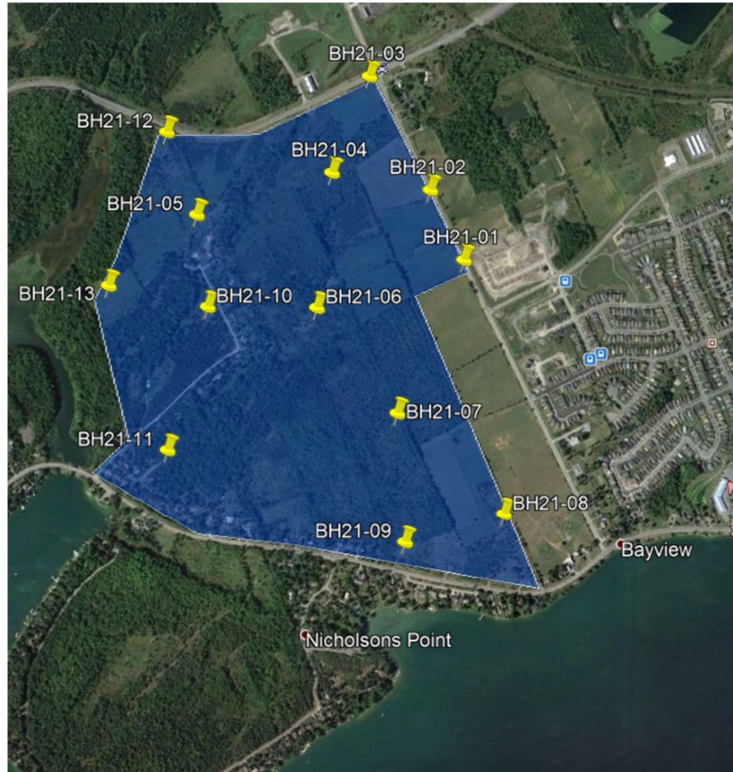
Figure 1: Survey Area with borehole locations marked
