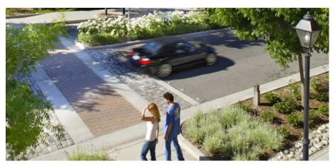
Figure 3.28 - Pedestrian Crossing as Traffic Calming Raised table crossing
